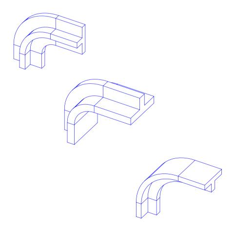
Sketch a section and a path as shown. (Avoid any constraints and dimensions between the two.)
